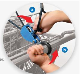
Easing tension on the ratchet release lever as illustrated will extend it's useful life.
