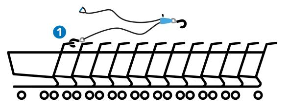
2 Place ratchet hook securely on the middle of the handle of the lead shopping cart.
